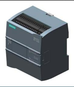
SIMATIC S7-1200, CPU 1211C, COMPACT CPU, AC/DC/RELAY, ONBOARD I/O: 6 DI 24V DC; 4 DO RELAY 2A; 2 AI 0 - 10V DC, POWER SUPPLY: AC 85 - 264 V AC AT 47 - 63 HZ, PROGRAM/DATA MEMORY: 50 KB
